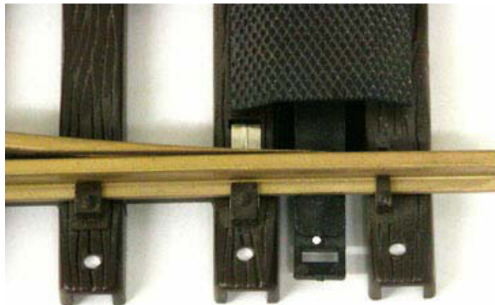
LGB turnout with new holes in tie end and tie bar.
